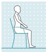
In a sitting position, i.e. when the thigh is close to horizontal and there is no load on the leg, the knee joint switches to low resistance in both the flexion and extension directions.
