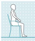
In a sitting position, i.e. when the thigh is close to horizontal and there is no load on the leg, the knee joint switches to low resistance in both the flexion and extension directions.
